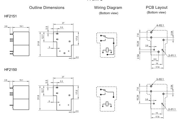
Remark: 1) In case of no tolerance shown in outline dimension: outline dimension ≤1mm, tolerance should be ±0.2mm; outline dimension >1mm and  $\leq$ 5mm, tolerance should be  $\pm$ 0.3mm; outline dimension >5mm, tolerance should be  $\pm$ 0.4mm.
