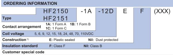
Notes: 1) We recommend dust protected types for a clean environment (free from contaminations like H2S, SO2, NO2, dust, etc.). We suggest to choose plastic sealed types and validate it in real application for an unclean environment (with contaminations like H<sub>2</sub>S, SO<sub>2</sub>, NO<sub>2</sub>, dust,etc.). If water cleaning is required after the relay is assembled on PCB, please contact us for suggestion about suitable parts.
