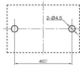
Remark: 1) In case of no tolerance shown in outline dimension: outline dimension  $\leq 1\text{mm}$ , tolerance should be  $\pm 0.2\text{mm}$ ; outline dimension  $> 1\text{mm}$  and  $\leq 5\text{mm}$ , tolerance should be  $\pm 0.3\text{mm}$ ; outline dimension  $> 5\text{mm}$ , tolerance should be  $\pm 0.4\text{mm}$ .
